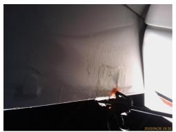
The patch material was of a similar type as the cover used originally. The patch were totally filled with T-88 epoxy and the fracture were held together with a clamp until the glue had settled. The left side picture shows the damaged area
