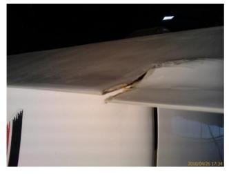
It was possible to glue inside both sides of the damaged area. Pressing T-88 epoxy inside for at least 50 mm from both sides, also adding a generous layer of glue on the carbon rod would ensure a strong bond.
