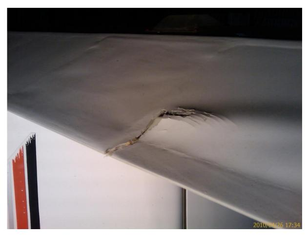
Since the TE consists of two wooden profiles in a V-shape, it has an internal opening of approximately 2 by 5 millimeter. A carbon fibre rod in that dimension was cutted in approximately 100 millimeter length. This will avoid the repair to break up again and add a lot of strength to the damaged area.
